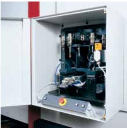
The linear axis transducers are the direct type in order to guarantee maximum accuracy and maintain this accuracy over time.
